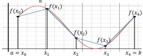
We then approximate the length of the curve for  $x_{i-1} \le x \le x_i$  with the length of the line segment connecting  $(x_{i-1}, y_{i-1}), (x_i, y_i)$ . That length is written as:
