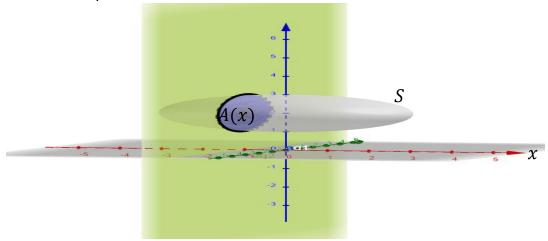
Now let's partition the x-axis into  $a=x_0 < x_1 < x_2 < \cdots < x_n = b$ , where the solid, S, lies between the plane that intersects the x-axis at x=a and x=b. Call  $\Delta V_k$  the volume of the solid S that lies between the planes that intersect the x-axis at  $x=x_{k-1}$  and  $x=x_k$ .
