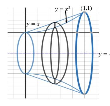
If we slice this solid with a plane perpendicular to the line y = -1, we will get annuli. However, we have to be careful when we calculate the inner and outer radii of the annulus.
